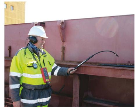
Testing for leaks by ULD
