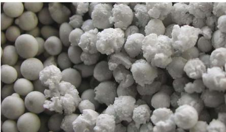
Distintegrated fertilizer due to water absorption
