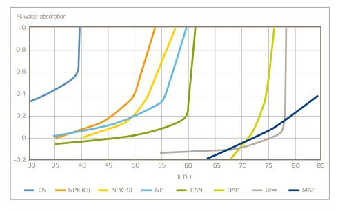
Hygroscopicity is an important property enabling prills and granules to dissolve quickly in the soil and thus supply nutrients readily to the plants after fertilizer application.
