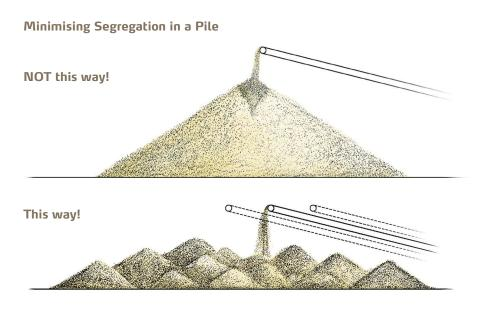
Segregation should be minimised through correct handling in order to avoid that a changing particle size distribution would induce deviating properties of the product.
