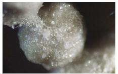
Crystal bridges between fertilizer particles cause caking
