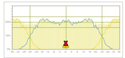
Spreading tables from the manufacturers of spreading machines are based on tests under ideal conditions in test stations, and give information on how to set the spreader for optimum even spreading at the desired application rate (kg/ha) and at a specific working width. The settings vary between machines and types of fertilizers. If spreading tables are not available, it is recommended to use field trial equipment to give an estimation of the spreading, although this method is less accurate.
