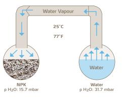
The water vapour pressure of the air varies with humidity and temperature of the air. Under tropical/summer conditions condensation may occur. This has an impact on quality of unprotected fertilizer stored in bulk.
