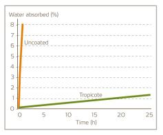
Yara has developed a unique coating for YaraLiva Calcium Nitrate that efficiently reduces the rate of water absorption.
