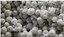
Distintegrated fertilizer due to water absorptior
