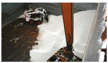
Correct bobcat driving during discharge operations avoids formation of extra fines and dust.
