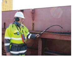
Testing for leaks by ULD
