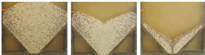
Poor quality blends segregate during handling
